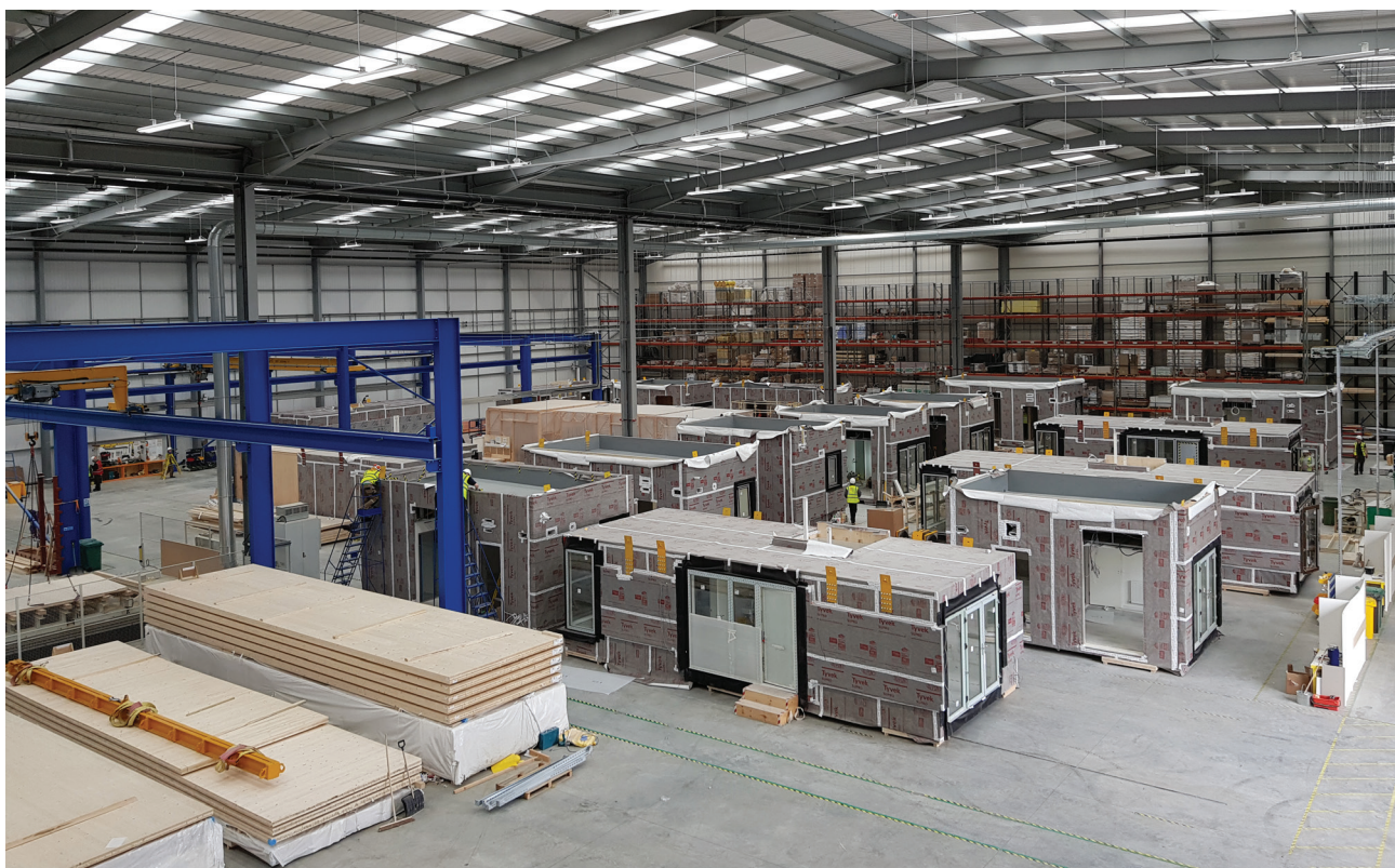
Volumetric modular factory showing the timber based units being finished with external membranes and windows
