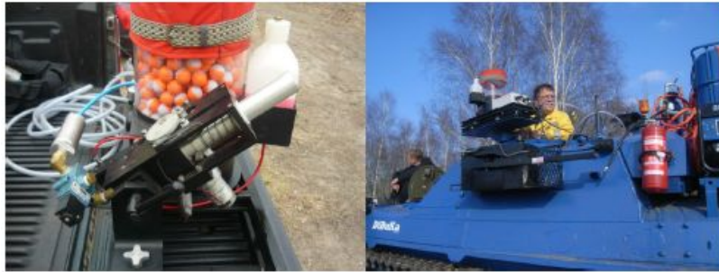
Fig. 11: Pyroshot Green Dragon (left and center) and the Foxfire Trail-Blazer ATV Drip Torch (right) mounted on the converted BMP OT-R5 (photos: project team).
