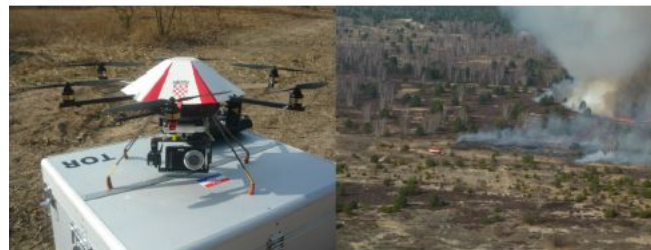
Fig. 13: The small octocopter drone type CT Bee 6B operated by project partner Crvena tipka d.o.o. (Croatia) provided realtime imagery (still photos and videos) of the prescribed burning operations allowing safe and precise ignition and suppression of escaping fire (photos: project team).
