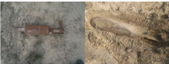
Fig. 8: Typical UXO recovered during clearing of the 7 m wide train surrounding the test site 10: (a) 125 mm shaped charge grenades; (b) light case explosive bombs (70 kg) (photos: project team).
